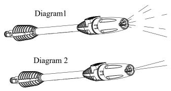
The adjustable nozzle will allow you to use any variety of spray patterns from a full fan spray (Diagram 1) to a direct stream spray (Diagram 2). When using the pressure washer to clean wood decks, siding, vehicles etc., always start using the fan spray and begin spraying from a minimum 36" away to avoid damaging the surface of the material you are cleaning. Always begin by spraying in a testing area free and clear of people and objects.
