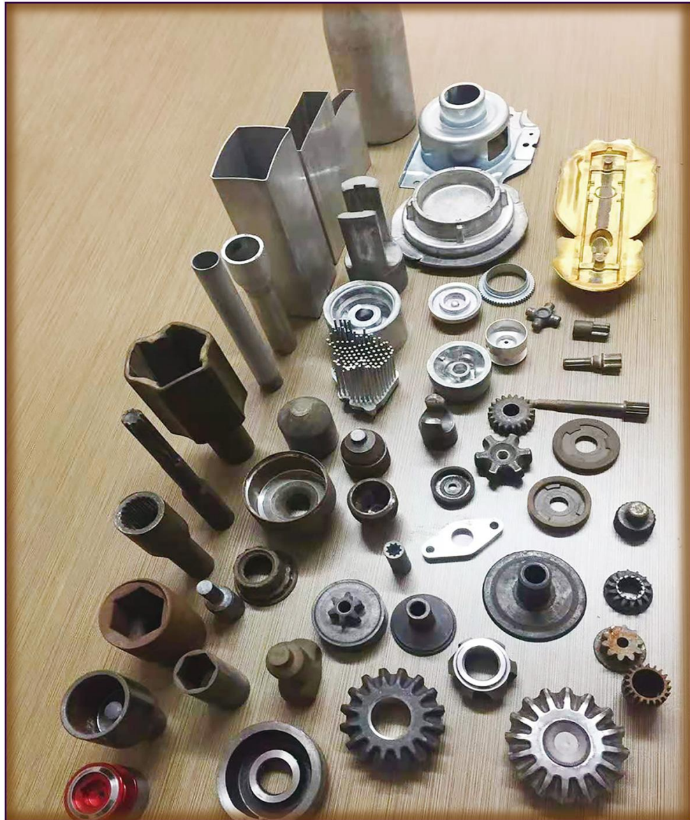
Cold extrusion molding hydraulic machine refers to the metal blank in normal temperature with the die through calendaring, stretching, pressing hole and other processes of the hydraulic press, especially suitable for aluminum and aluminum alloy products cold extrusion and temperature extrusion molding.
