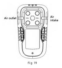
During calibration, the air inlet on one side of the cover is connected to the span gas through ahose. The other side is used as an air vent.
