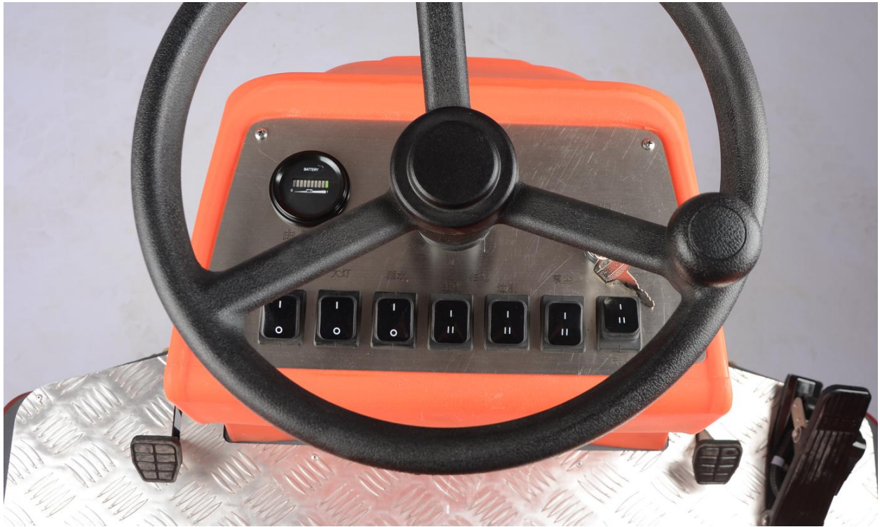
(1) power switch (2) horn button (3) forward backward switch (4)floor sweeping switch (5)LCD instrument assembly (6)steering
