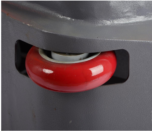
(三) Side brush anti-collision mechanism
