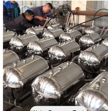
Water Pressure Test
