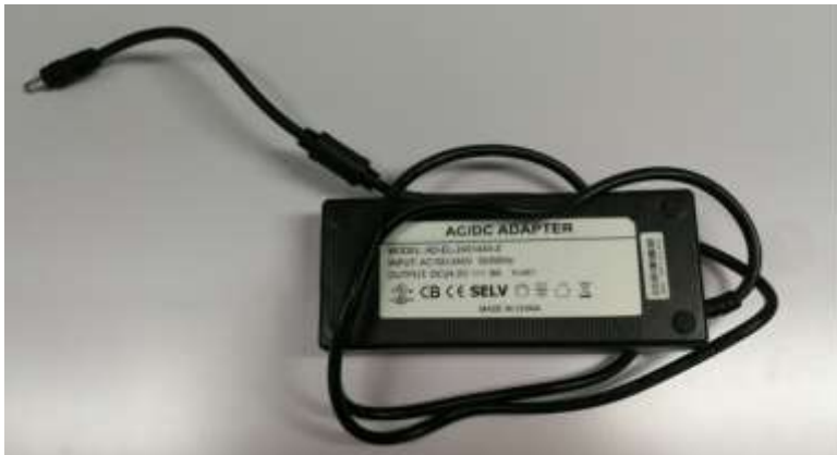
Power adapter: 144W This adapter can drag three sets of light strip
