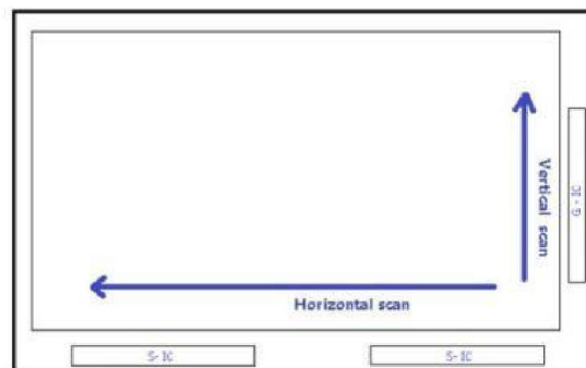
Fig. 2 Reverse scan (Pin24, Reverse = High)
