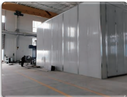
Purpose: Sandblasting Process Range: 2500x6000x2500
