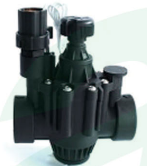
YH-CT119B 1.5 Inch Solenoid valve Pressure:0.10~1.04 MPa Flow rate:0.45~34.05 m3/h water temperature:≤50℃ Environment temperature:≤80℃
