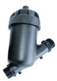
YH-CT121A 1 Inch Inline Filter Maximum operating pressure:6kg/cm2 Flow:333 L/minute or 20000 L/Hour
