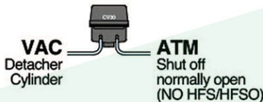
YH-ME133A CV30 Operating Voltage: 12/24VDC Power Consumption: 540mA (270mA for solenoid 12V) 260mA (130mA for solenoid 24V) Vacuum Ports: 2 Exits
