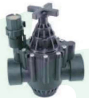
YH-CT119A 2 Inch Solenoid valve Pressure:0.10~1.04 MPa Flow rate:0.45~34.05 m3/h water temperature:≤50℃ Environment temperature:≤80℃
