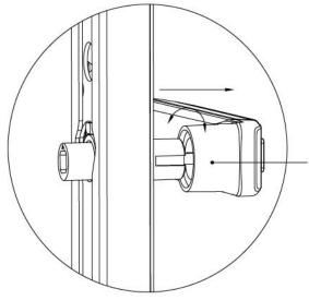
The handle will be gently removed, and then switch 180° direction (you can first press the screw to low and then observe whether the screw is pressed fingerprint head data line and then tighten the screw after the handle is installed)
