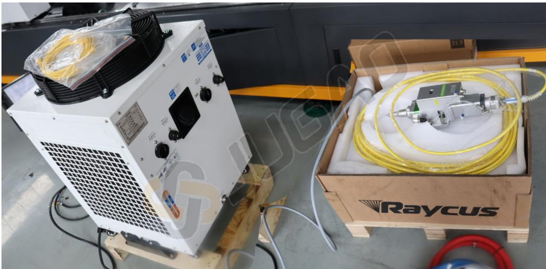
water cooler. / Laser cutting head
