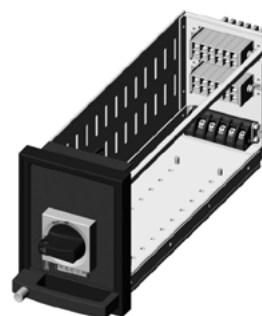
The drawer solution satisfies the subway signal control cabinet, satisfies the main circuit 10A, 6 contacts, and satisfies the auxiliary circuit 24 contacts
