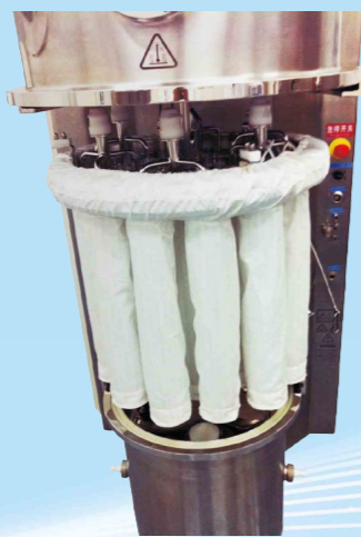
下料管 Tube 顶指 Stopper Finger 字钉 Coding Number/Letter 滤袋 Filter Bag
