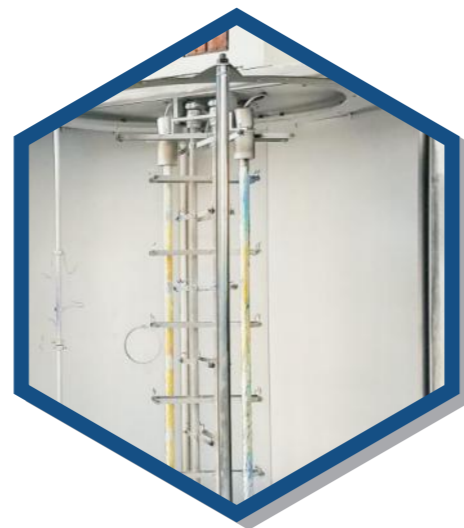
>高效镀透式设计蒸发源< High efficient Cross-coating source design
