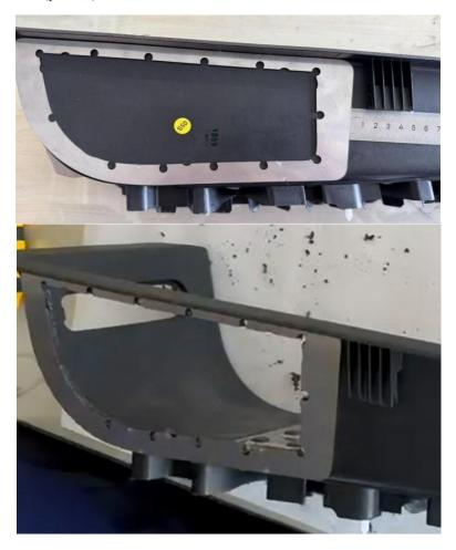
• Install the front step intake panel and front step intake bracket to the **front step trim panel** using eleven M3\*6 self-tapping screws and flat washers.
