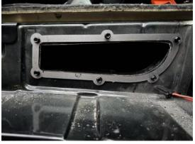
• Connect Upper Air Channel Guide and Lower Air Channel Guide (part ⑥ & ⑦), then fix them onto the B-pillar reinforcement panel opening with outlet Frame (Part ⑤) using two M5\*20 self-tapping bolts.
