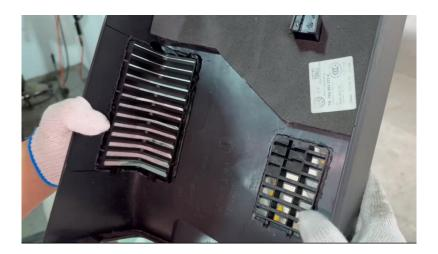
• Connect T5/6 Air Guide (part4) to the T5/6 Frame(part5)[snap on]
