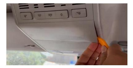
Pass the **controller branch** through the floor near the right passenger seat. Route vertically along the A-pillar to the overhead console cavity.
