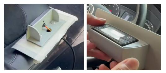
• Connect the controller wire to the harness and put the trim panel back.
