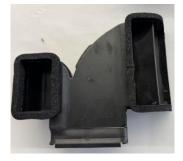
• Install Rear B-Pillar Vent (Part①) & flat air vent (Part②) on the B-pillar trim panel [snap on]
