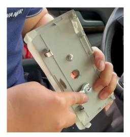
• Thread the controller's wire through the circular hole, then apply 3M double-sided tape to the back of the controller, and attach the controller to the bracket. Snap the bracket into the bracket base (Part 17).
