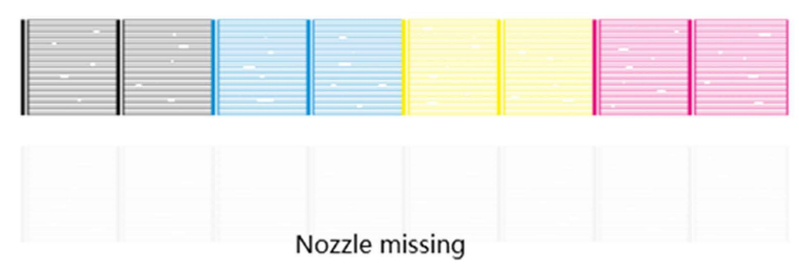
Some nozzle missing is due to is caused by ink corrosion or volatilization. Automatic cleaning can be solved at this time. If automatic cleaning can not be solved, it can be printed normally, which does not affect the printing effect.
