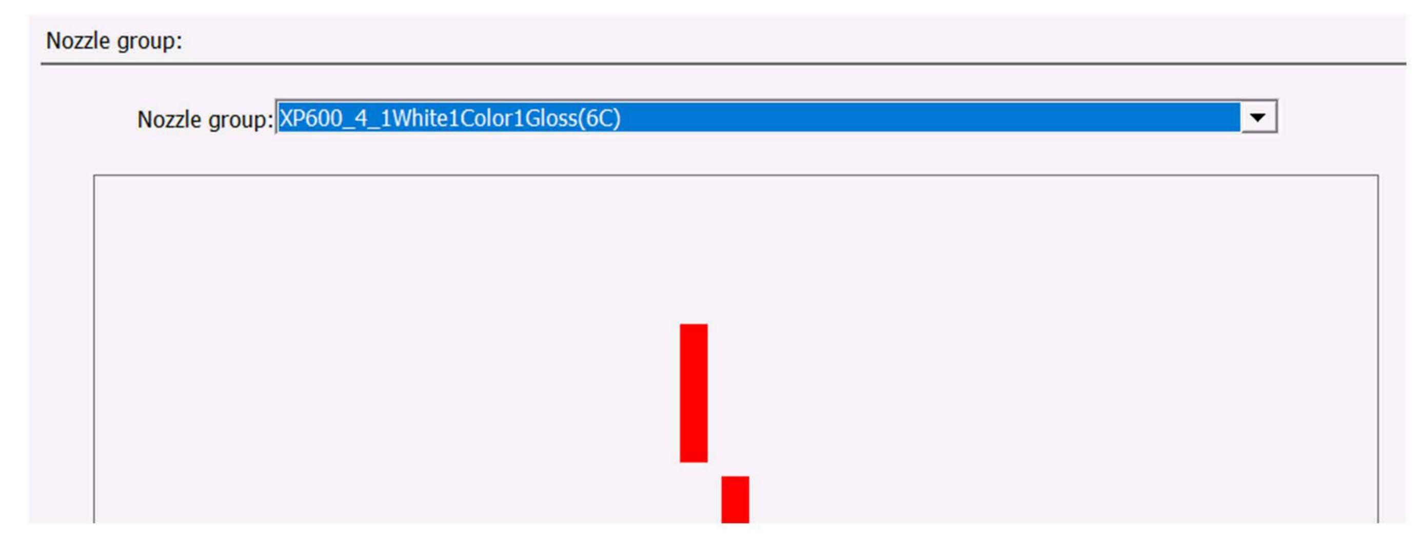
Set the printhead combination according to the physical location of the head.
