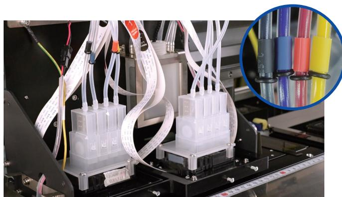
Note: the ink sac holder is installed first, and the ink tube is connected to the ink sac. The ink sac installation position is required. The color ink is on the left printhead, the installation sequence is k c m y, and the right side is white ink
