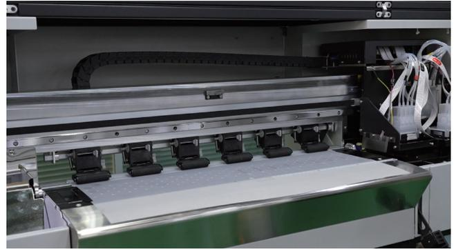
Note: loosen the screw on one side of the paper feeder and place the printing material in the center to fix. Lift the back roller handle, feed the material and press down. Lift the front roller handle, check whether the material is perpendicular to the horizontal direction and no wrinkles, and press down without problems
