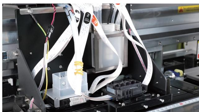
Note: data cable installation has the direction and position requirements, according to the data cable labeling installation
