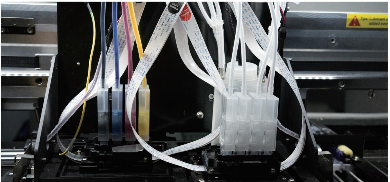
When not used for a long time, you need to open the software to fill ink to clean the print test strip every two to three days. Ensure that the whole path is full of ink, to prevent clogging the printheads
