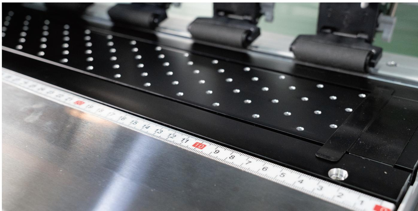
Keep the platform clean to prevent the contaminants from damaging the print head or affecting the printing.
