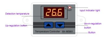
Installment pitch of holes:73MM (hole pitch 4MM)Panel introduction
