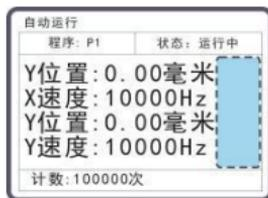
In this mode, press the [Run pause] key to run the program. The display status bar displays [running] and press again
