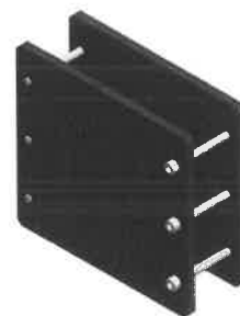
Fig. 2 Diagram of the clamp covered with insulation film 图 2 电池夹具包绝缘膜图
