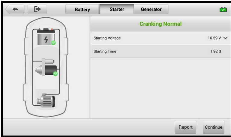
Figure 12-8 Starter Test Result Screen
