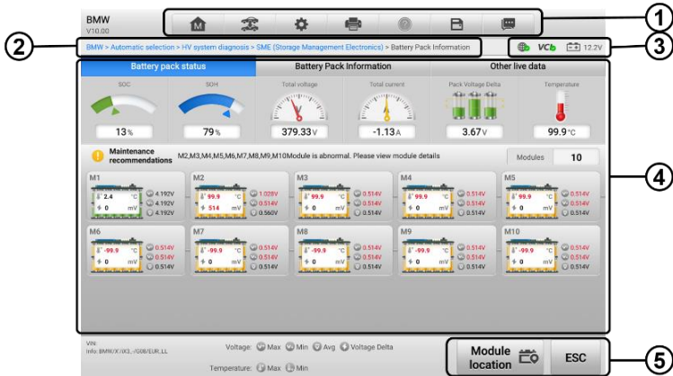
Figure 4-22 Battery Pack Status Screen
