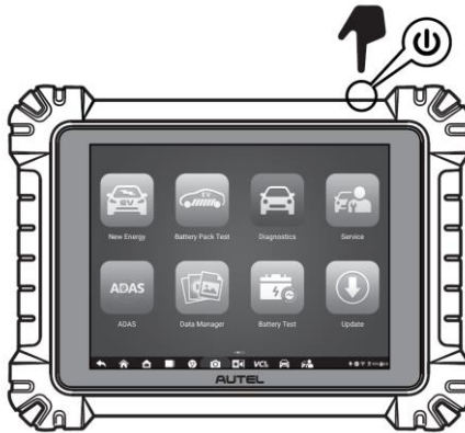
Figure 5-3 Power up the Tablet
