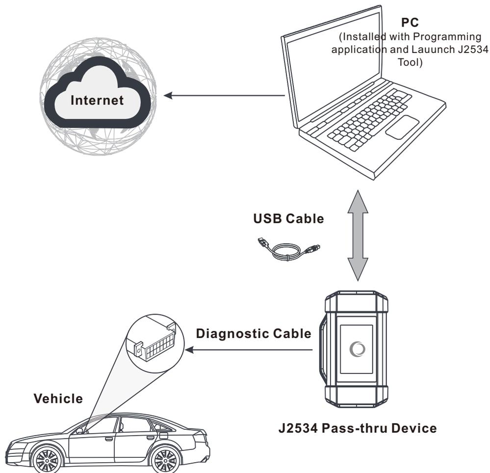
2. Run the vehicle manufacturer's programming application on the PC.
