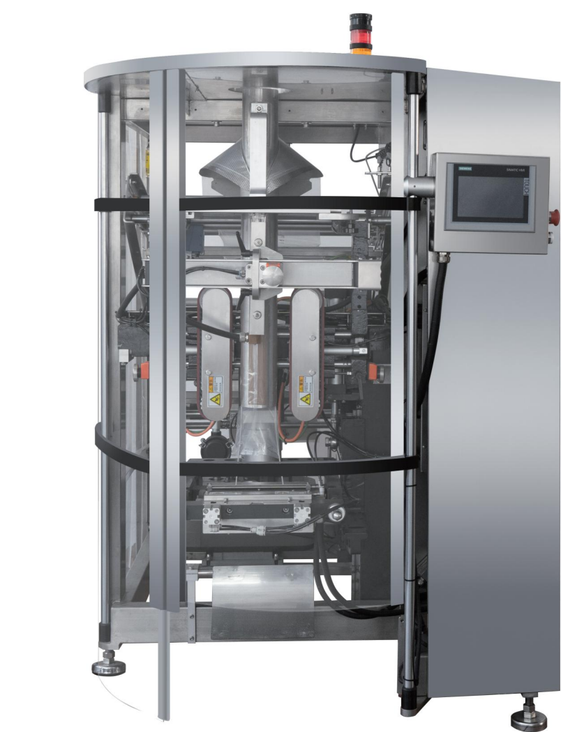
背封间歇式立式机 (中小袋型/中大袋型) Back sealed, intermittent machine (Small bag/Large bag)
