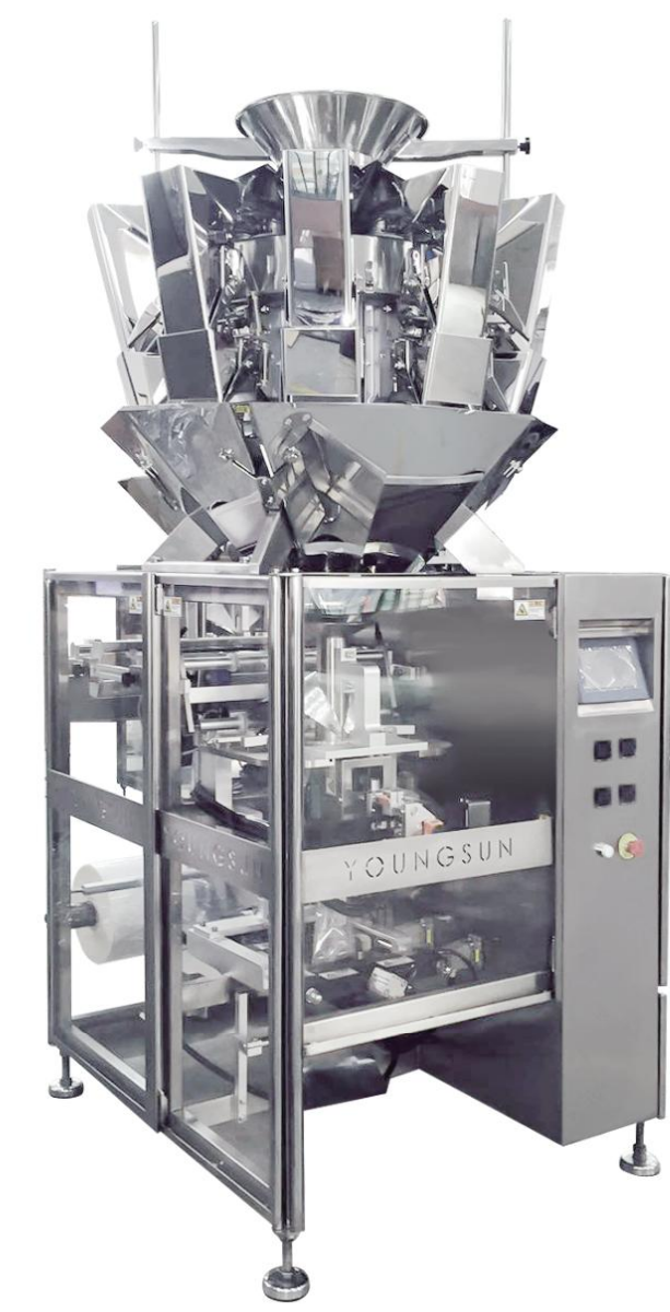
组合秤包装一体机 Combination MHW & packaging machine
