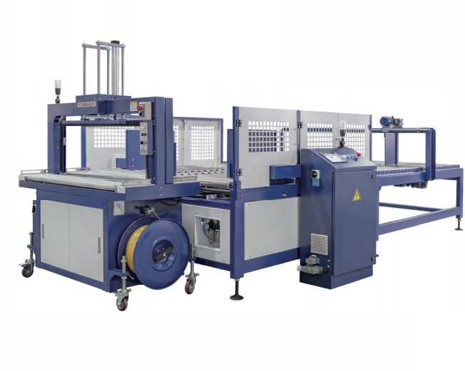
YS-LX-500 全自动拢箱装置 Automatic corrugated bundle squaring device
