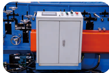
PLC 控制柜 PLC Control Cabinet
