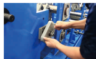
2. 旋转180度 Rotate the adjustment tool 180 degree
