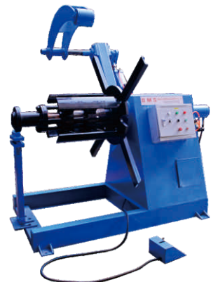
5吨液压放料机带压紧臂 5 Ton Hydraulic Decoiler With Clamp Arm
