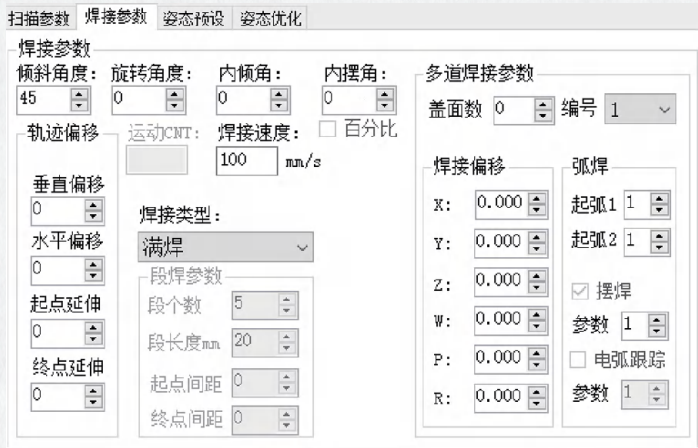
Full Welding, Segment Welding, Spot Welding, Weaving Welding, and Arc Tracking Parametric Configuration
