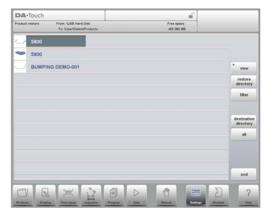
In the restore screen the products in the selected directory are shown. Basic functions to change the view can be chosen similarly to the Products mode. This enables to easily find the required products to be restored.
