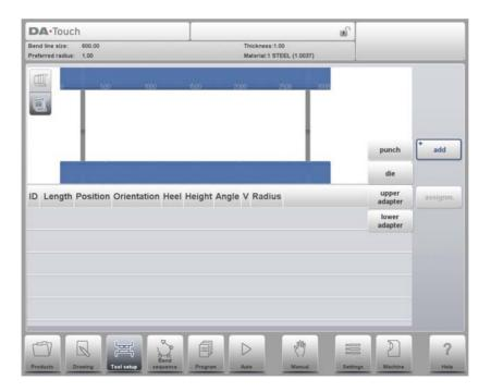
When a tool has been chosen (e.g. a punch), it is placed in the machine with maximum available length.
