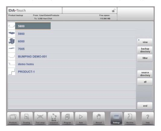
In the backup screen the products in the selected directory are shown. Basic functions to change the view can be chosen similarly to the Products mode. This enables to easily find the required products to be backupped.
