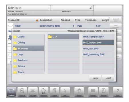
For the DXF file to be imported it is advised to create the original drawing as accurate as possible. Bend lines should be connected to contour lines to obtain an accurate product drawing. If this is not the case, the DXF Converter can correct small errors.
