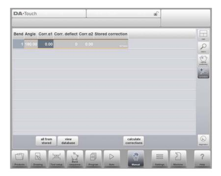
The programmed corrections can be verified here similarly to the corrections in Automode. Entries in the correction database and for initial correction can also be monitored in this screen. Since these are of significant influence on the bend result, access to the database can be used to modify. This can also be usefull while finding appropriate corrections with testbending and storing the found results in the database.
