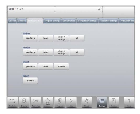
The actual backup directory consists of a device (USB disk, network) and a directory. The choice of devices depends on which devices are connected to the control. If necessary, directories can be created and selected. The backup locations for storage of products and tools are set independently.
