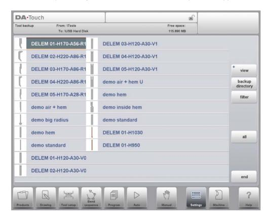
With this menu a back-up of tools on the control can be made: punches, dies or machine shapes. The procedures for a tool back-up run similar to the procedures for a product back-up.
