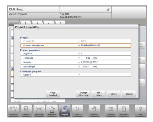
The main screen shows the existing numerical program or, when starting a new program, the first to be programmed bend.
