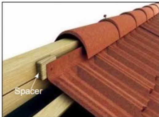
Option 2: Ridge batten with spacers
