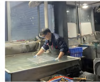
Air Tightness Testing
