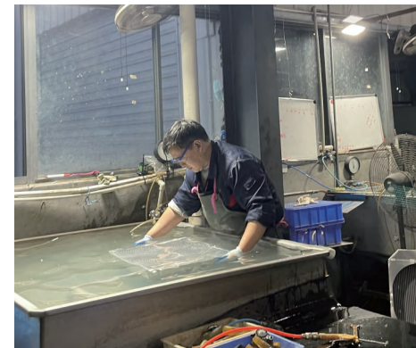
Air Tightness Testing
