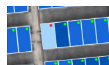
Shutdown one module
