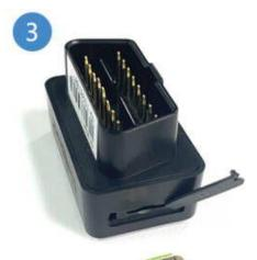
Insert SIM card with chip facing upwards
