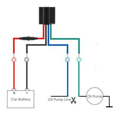
NOTE: Working voltage: 10-40V DC, please find professional repair man or 4S store to install the device!
