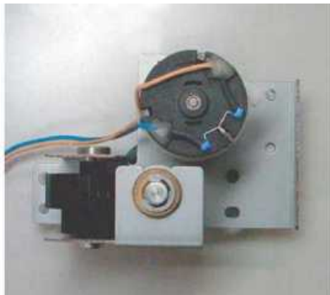
Figure 5 Stacker motor installation
