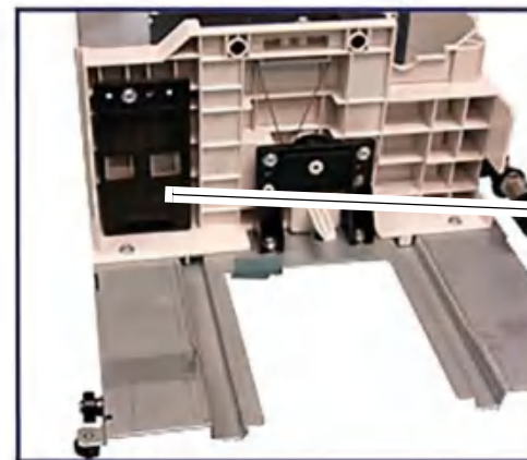
Figure 13 Tray 3 paper size sensor actuator
