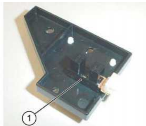
Figure 4 Rear tamper home sensor removal
