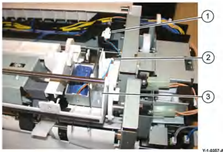
Figure 1 Sub paddle solenoid assembly removal
