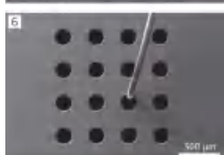
钢中的 200 μm 钻孔, 与头发丝对比, 固定工件位置, 无 XY 平移台 (SEM 图像) 200-μm bore holes in steel – compared to a human hair, fabricated with fixed workpiece position, without an XY translation stage (SEM image)
