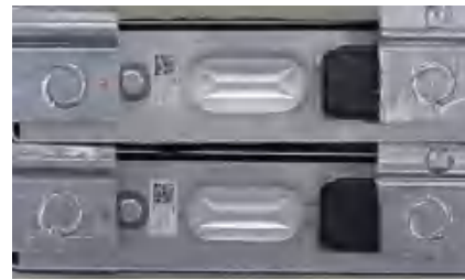
汇流排焊接 Busbar welding
