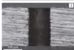
直径为 100 μm 的孔的横截面, 垂直壁厚为 200 μm 的钢轮廓 (零锥度), 处理时间 1 s Cross section of a 100-μm diameter bore hole in 200-μm thick steel with perpendicular wall contour (zero taper), process time 1 s
