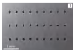
厚度为 300 μm 薄板的灵活几何形状 (SEM 图像, 出口侧) Flexible geometries in 300-μm-thick steel (SEM image, exit side)
