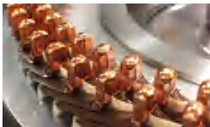
扁铜线焊接 Hairpin welding
