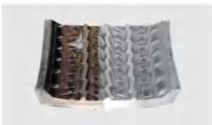
轮胎模具清洗 Tire mold cleaning
