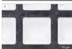
4 x 4 方孔阵列的细节在陶瓷中 - 方形几何尺寸: 30 μm x 30 μm - 深度: 300 μm - 长宽比: 1:10 - 垂直壁轮廓 - 圆角半径: <4 μm - 壁厚: 10 μm (SEM 图像) Detail of a 4 x 4 square hole array in ceramic - Square geometry: 30 μm x 30 μm - Depth: 300 μm - Aspect ratio: 1:10 - Perpendicular wall contour - Corner-rounding radius: < 4 μm - Wall thickness: 10 μm (SEM image)
