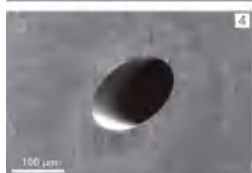
图 1 的细节: 椭圆孔, 长 190 μm, 宽 110 μm (SEM 图像) Detail of figure 1: Elliptical bore hole, 190 μm-long, 110 μm-wide (SEM image)
