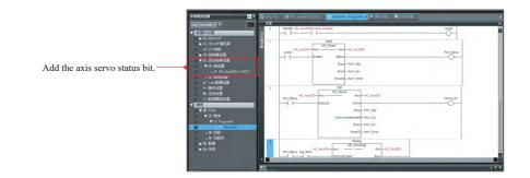
② After the configuration and programming are complete, click the compile controller  $\mathbf{k}$ , switch the controller back to the online state, and click  $\mathbf{k}$  to download the program to the controller.
