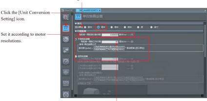
Set [Display Unit] according to the actual running unit of the load.
