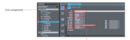
Axis number: Number of the servo Ethernet communication station, value of C13.01
