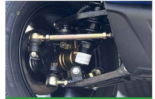
Front Double Wish-bone Independent Suspension
