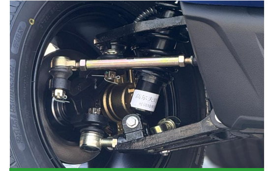
Front Double Wish-bone Independent Suspension
