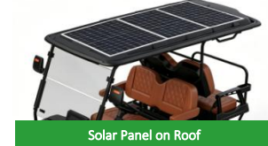
Solar Panel on Roof
