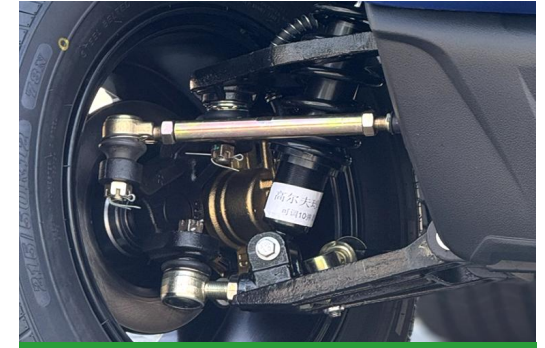
Front Double Wish-bone Independent Suspension
