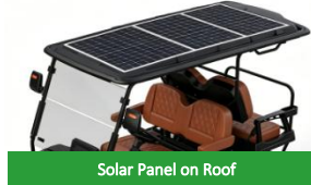
Solar Panel on Roof
