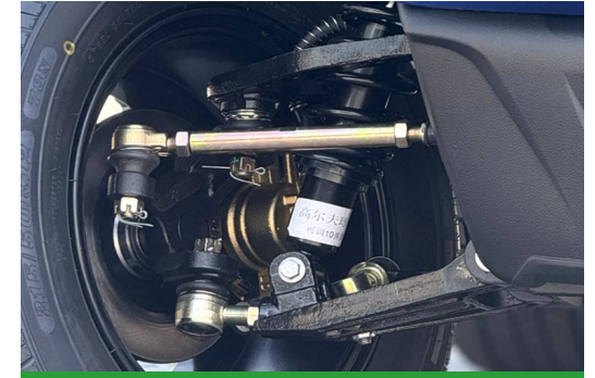
Front Double Wish-bone Independent Suspension
