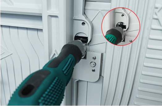
Turn the module lock 90 degrees clockwise to open it
