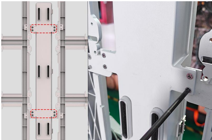
Remove the 8 fixing screws of the power box
