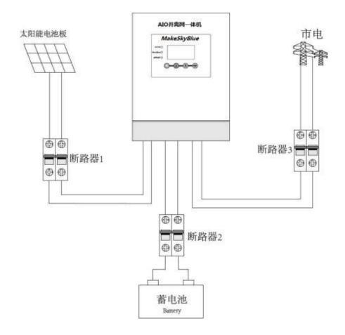
Utility AC, battery, solar panel input will require the installation of circuit breaker, circuit breaker specifications are as follows:
