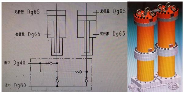
6. Servo Pressure Intensifier Cylinder for Wellhead Injection UCZ1902JKZSWL12L-ZYG UCZ1902JKZSWL12L-ZYG (Servo Intensifier Cylinder)
