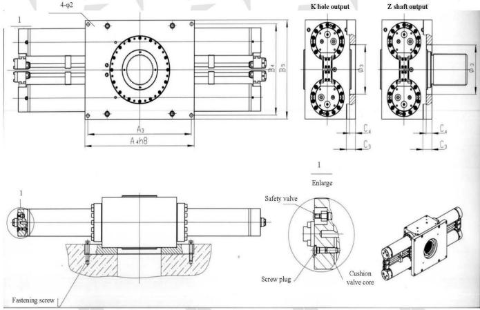
Note: The four fastening screws are not designed to withstand torque. Torque transmission must be borne by both A4h8 side surfaces.
