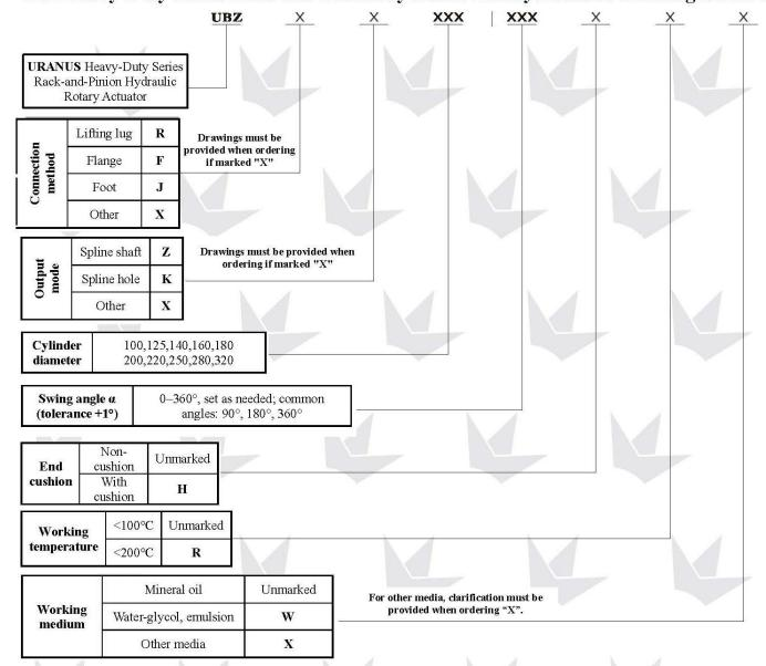
Selection Example: required torque: 180,000 Nm; system pressure: 20 MPa;  $K_1$  = 180000  $\div$  (20 - 1)  $\approx$  9474; cylinder diameter size:  $\phi$  = 180 K >  $K_1$ ; mounting method: flange-mounted, hole output; swing angle: 220°; with end cushion; operating temperature 120°C; working medium: hydraulic oil; marking: UBZFK180/220°HR
