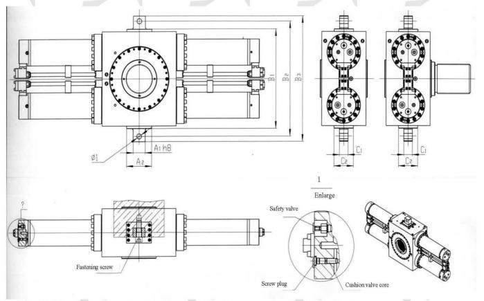
Note: The two fastening screws are not designed to withstand torque. Torque transmission must be borne by both A1h8 side surfaces.
