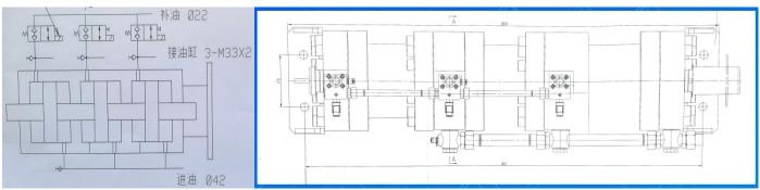
3.Synchronous Distributor Hydraulic Cylinder UF4 \$\Phi\$ 200/90-200LH
