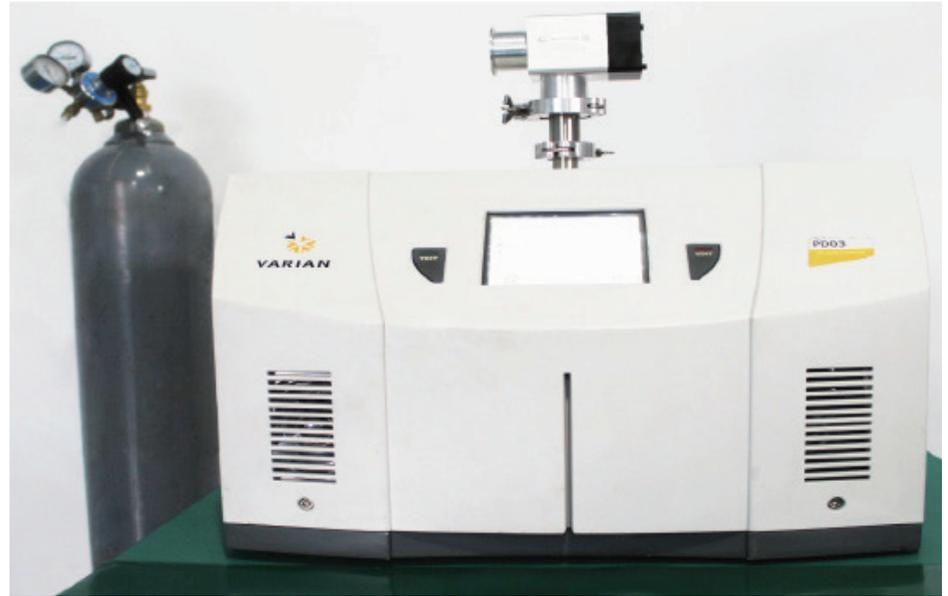
Helium Mass Spectrometer Leak Detector
