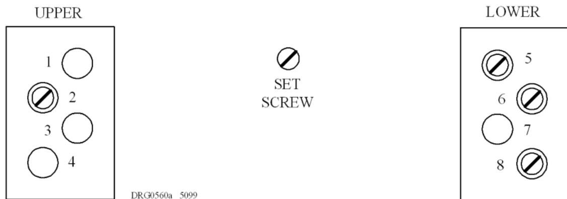
Figure 2-1 Chassis mechanical coding block configurations
