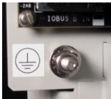
Figure 2-29 Protective Conductor Terminal
