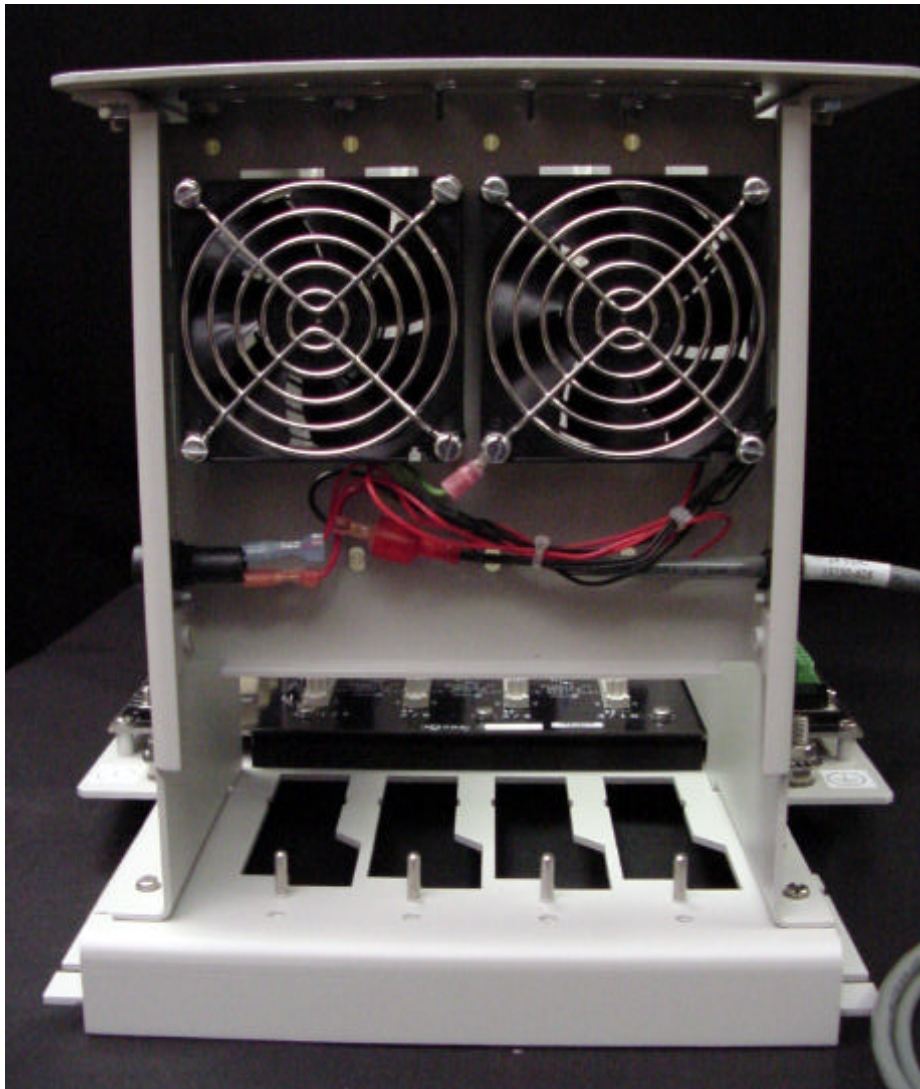
Figure 2-26 Bottom View of Rack Showing Built-in Recirculating Fans
