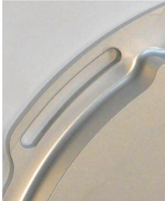
FIGURE 2: Close-up view of slotted mounting holes in HSCT housing
